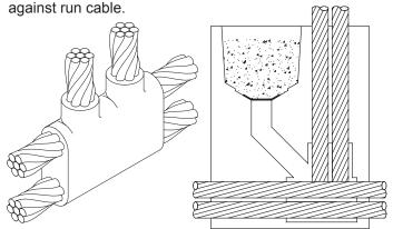
Place run cables into mold. Butt tap cable against run cable.
